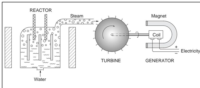
Figure 9: Boiling Water Reactor Nuclear Power Plant
