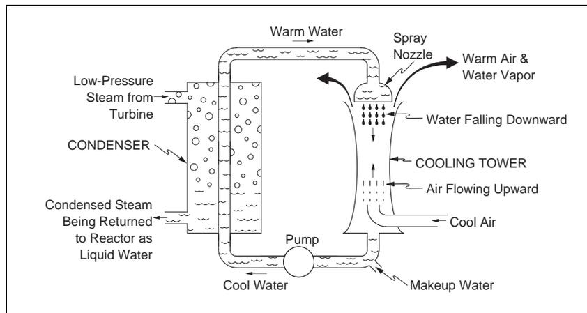
Figure 11: Cooling Tower
