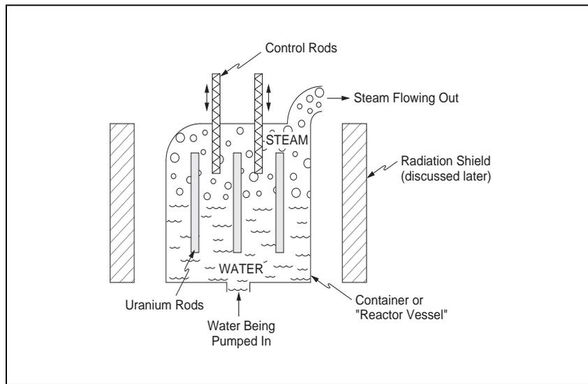
Figure 5: Boiling Water Reactor
