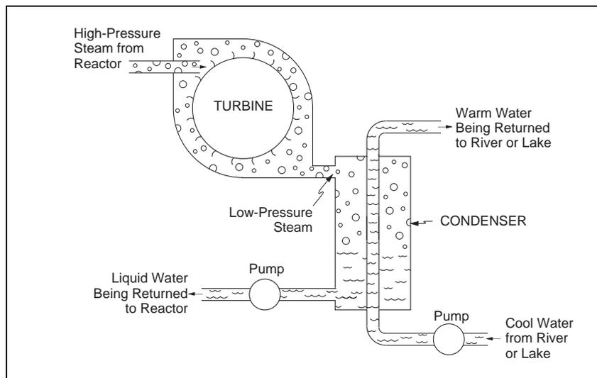
Figure 10: Turbine and Condenser
