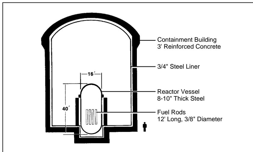
Figure 13: Pressurized-Water-Reactor Containment Barriers
