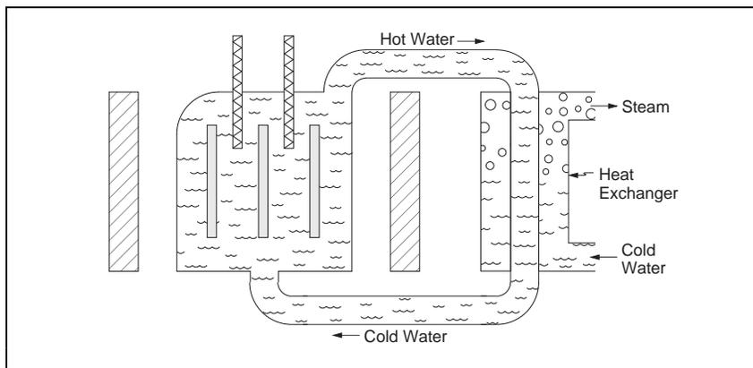
Figure 6: Pressurized Water Reactor
