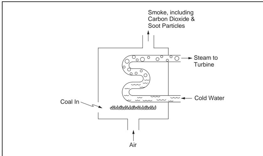
Figure 12: Coal Plant Furnace
